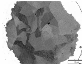
**The soft phase is more than 1000 times as large as the upper size limit predicted by the current model of exchange coupling**
